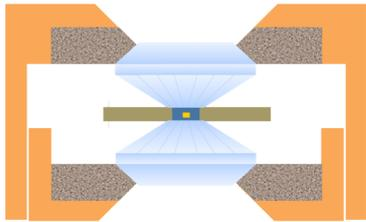
The protein crystals in the sample chamber will be compressed with the uniform hydrostatic pressure generated by the squeezing of the chamber volume between the two diamond's culets.
