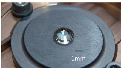
One of the key tools of HPPX is a pressure-generating device, DAC.
