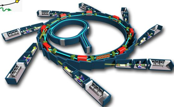
With this ring structure, we can make several experimental "stations" around the ring.
