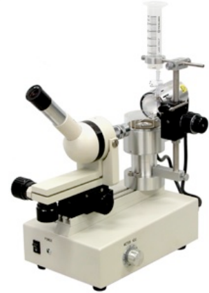
micropipette grinder (Narishige EG-400)
